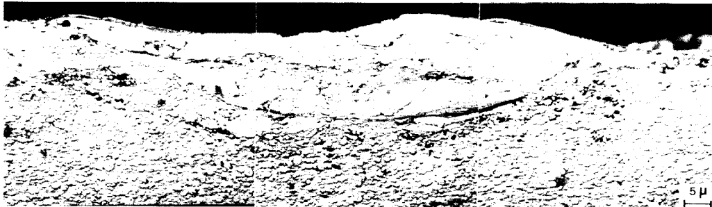
Fig. 15. SEM micrograph of cross sectional view of damaged pin showing white etching area(nital etch).
