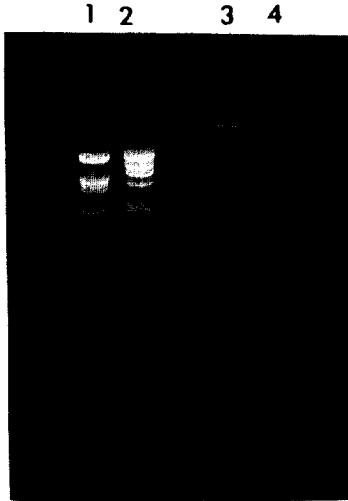
Fig. 1. Gel electrophoretic pattern of plasmid DNA in JM 109 strain. lane 1: Hind III + Eco RI double-digested DNA. lane 2: Hind III digested \lambda DNA. lane 3,4: cDNA of PNMT gene fragment cloned pBR 322. Electrophoresis was carried out at 50 V for 1 hr in 1% agarose gel.
