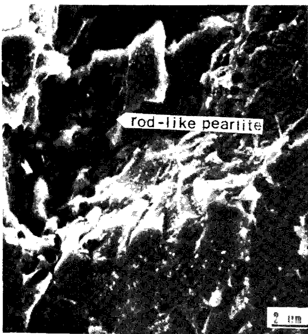
Photo. 4 SEM microstructure of the \gamma Fe solid solution transformed to rod-like pearlite.
