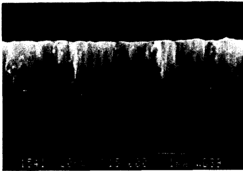
Photo. 1. Scanning electron micrograph of cross section of the TiN deposited on Si-wafer by PACVD; (Temp., 500 C; deposition pressure, 2 torr; total flow rate, 200 sccm; r.f. power, 70 W; electrode distance, 3 cm; gas inlet fraction, TiCl 4 /N 2 /H 2 /Ar=0.01/0.4/0.25/0.34)
