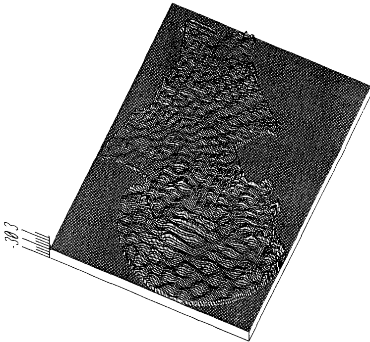
Fig. 12 Surface Pattern for Pusan Harbor (30sec, ESE direction, K_r=0.8 , \beta=0.0 , open end)
