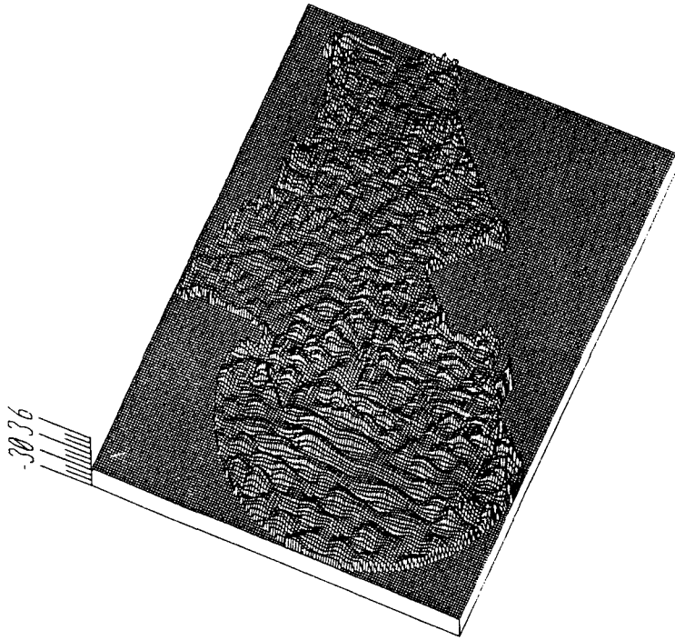
Fig. 11 Surface Pattern for Pusan Harbor (30sec, ESE direction, K_r=0.9 , \beta=0.0 , open end)
