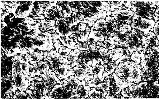
(a) t_{\text{on}}=0.1\text{ms} , 40^{\circ}\text{C} i_m=1\text{A}/\text{dm}^2 , i_p=100\text{A}/\text{dm}^2
