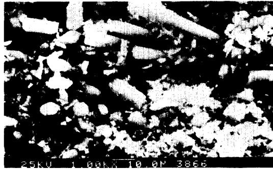
Fig. 10. Micrographs of the massive failure region.
