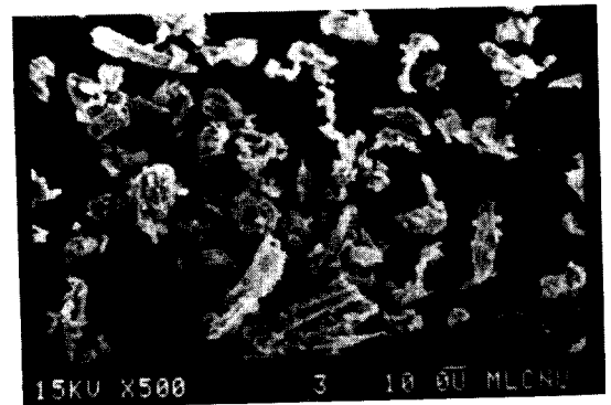
Fig. 3b. Electron microscope photos of ligno-cellulosic material. (AFEX-treated rice straw)
