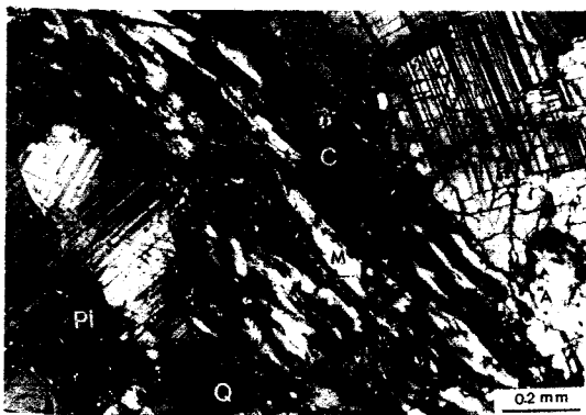
Fig. 2a) Photomicrograph showing alteration of amphibole (A) to chlorite (C) and muscovite. (M) Pl: Plagioclase, Q: Quartz.
