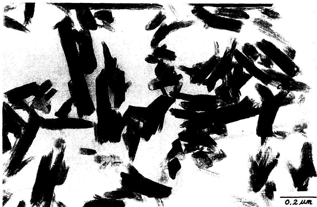
Fig. 5. Transmission electron micrograph of the finest fraction (No.3 in Fig. 3) shows halloysite tubes with various length and thickness.
