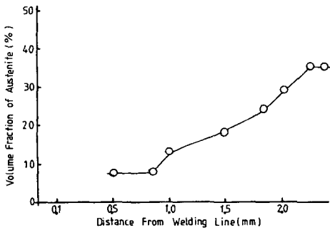
Fig. 2 Change in volume fraction of austenite in welding zone
