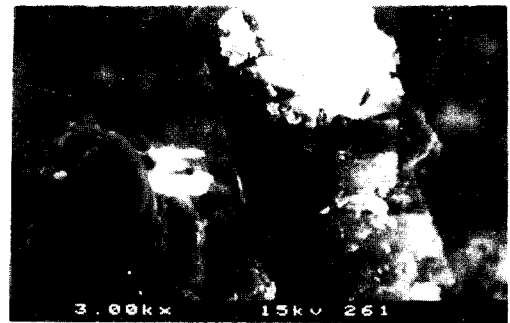
Fig. 15 Fractography of fiber debonding from matrix ( \times 3000 )
