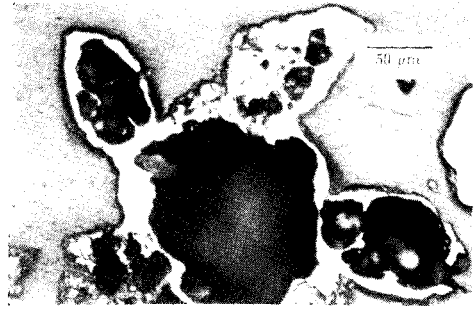
Fig. 7 Cross-section micrograph of Char prepared following the procedure of typical proximate analysis (i.e. 7min. heated at 1200K)
