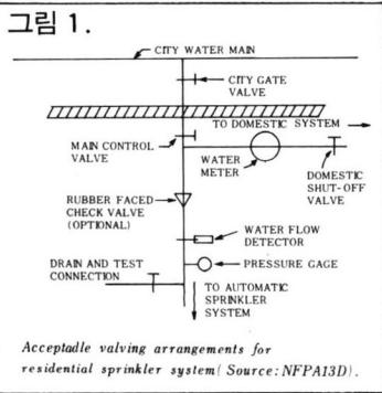
*Acceptable valving arrangements for residential sprinkler system (Source: NFPA13D).*
