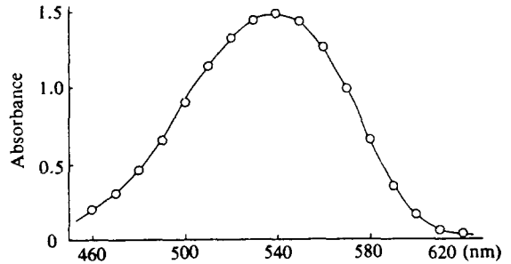
Fig. 5. Absorbance spectra of azo dye formed from the diazo-coupling reagent dissolved 30% acetic acid solution.
