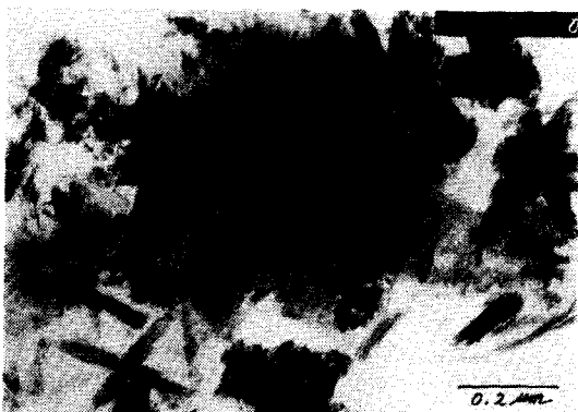
Fig. 3. TEM photograph of goethite concentrate prepared by 5M-NaOH method. Note the acicular goethite crystals.
