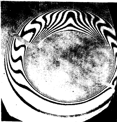
Fig. 5 Interferogram taken using air for Ra_L=2.43 \times 10^4 , Pr=0.704 at lying position
