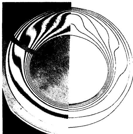
Fig. 7 Comparison between experimental and numerical isotherms for Ra_L=1.44 \times 10^4 , Pr=0.706 at lying position
