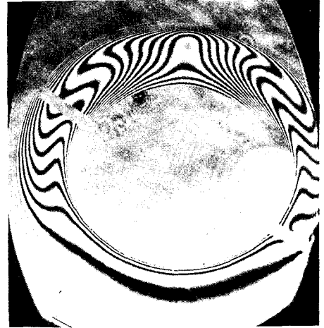
Fig. 6 Interferograms taken using air for Ra_L=3.076 \times 10^4 , Pr=0.702 at lying position
