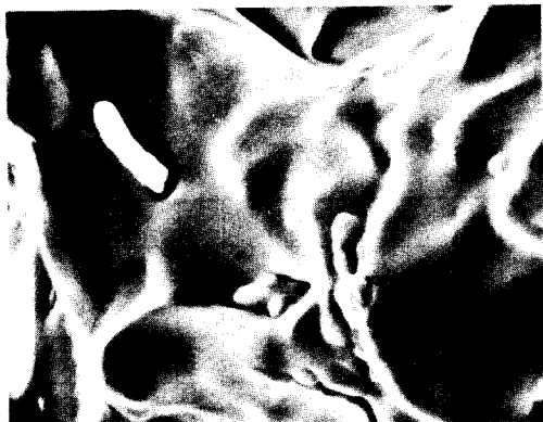
Photo. 2 Typical fracture surface in heat OA1090 (303) tested on-heating to a ZDT of 2500°F(SEM5000x).
