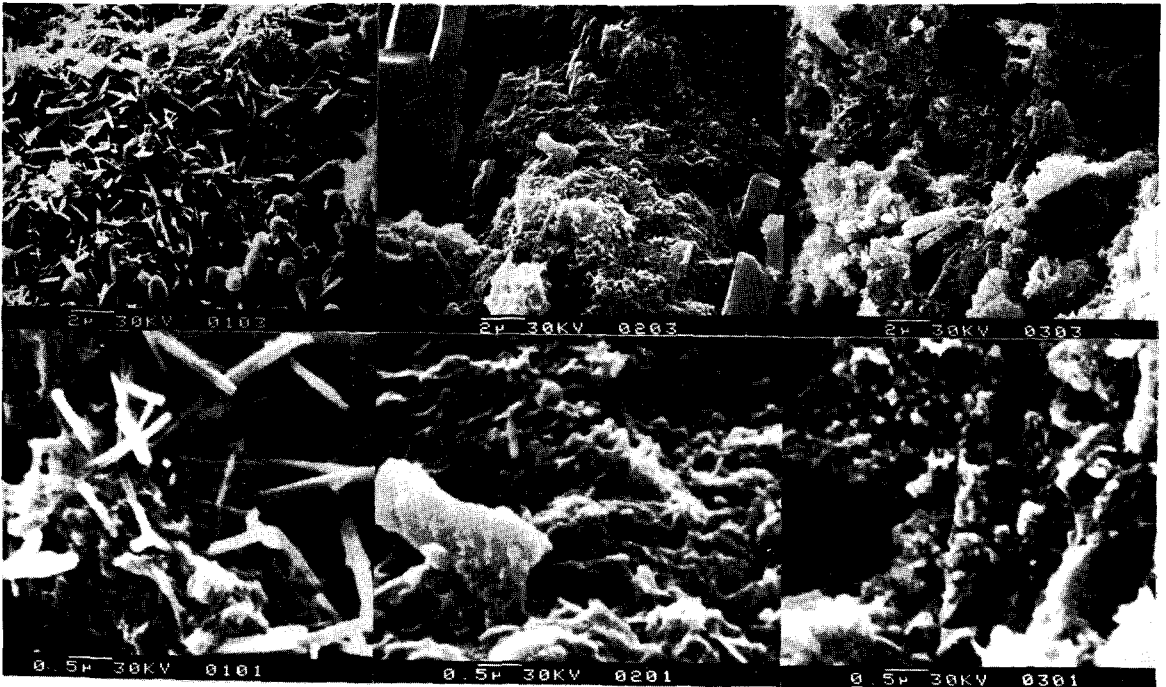
〈그림-7〉 SEM-Micrographs of Hardened Portland Cement Paste with and without Concrete Admixtures after 28-Days Curing. From left Zero-, Fructose (0.60%)- and Starch (1.00%)-Paste
