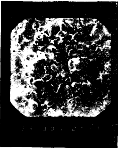
Fig. 7. SEM of Vita VMK 68 A 1 opaque. (Magnification × 1000)
