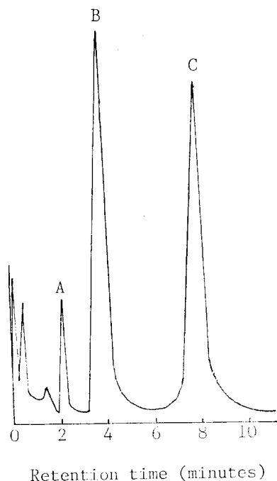
Fig. 1—Head-space gas chromatogram of rat blood after extraction with thiourea, perchloric acid and sodium azide. Coiled glass column 1.8 \times 2mm I.D., porapak Q(100-200mesh). A=acetaldehyde, B=ethanol, C=isopropanol(internal standard).
