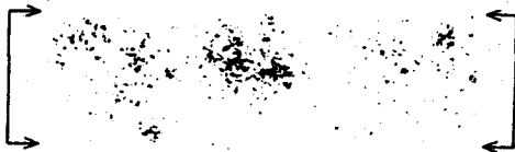
(e) Lubricated copper laurate. Pick-up 10^{-9} gm. cm.
