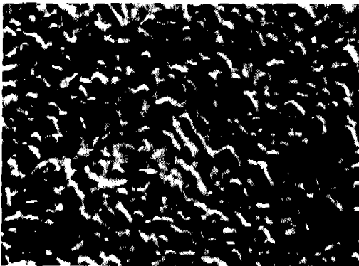
Fig. 11 SEM Micrograph of Deposit Collected from Flame Doped with 100% Saturated \text{K}_2\text{SO}_4 Aerosol
