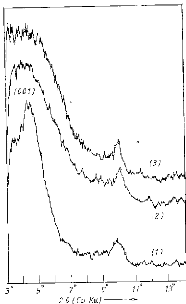
Fig. 5. X-ray diffraction patterns of PVA intercalated montmorillonite, (1) PVA 500, (2) PVA 1000 and (3) PVA 2000, reacted for 76 hours
