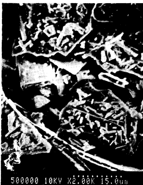
Fig. 1d —Scanning electron micrograph of phenylbutazone deposited on 90% (w/w) dibasic calcium phosphate (2,000 \times ).
