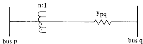
Fig. 2. Convention of off-nominal tap of LTC.
