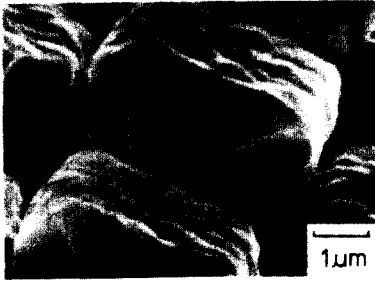
Photo 1. Defects appearing in metal films over unflown steps. Microcrack, concave etch defect and capillary tunnel are shown by arrows.
