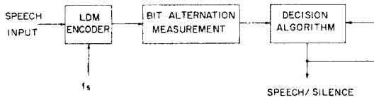
Fig. 3. Block diagram of the silence/speech detector.
