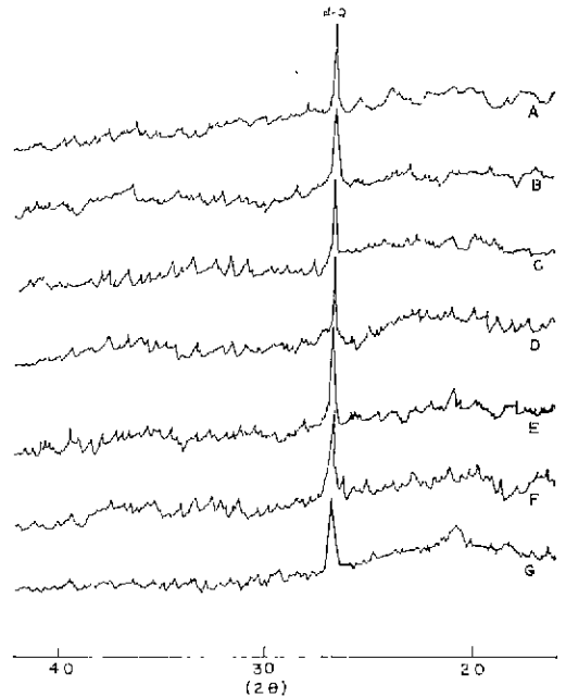
Fig. 4 X-ray diffraction patterns of fluoride-added specimens (950°C-2hrs. 0.2wt% on the basis of fluorine)
