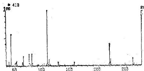
Fig. 8. Mass spectrum of metabolite V, N-[4'-(4-chloro-phenoxy)] phenyl acetamide
