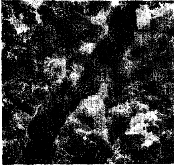
PLATE 6. Scanning Electron Micrograph of a Crack in Closed-up in the Middle Left Part of # 4-A, Plate 6
