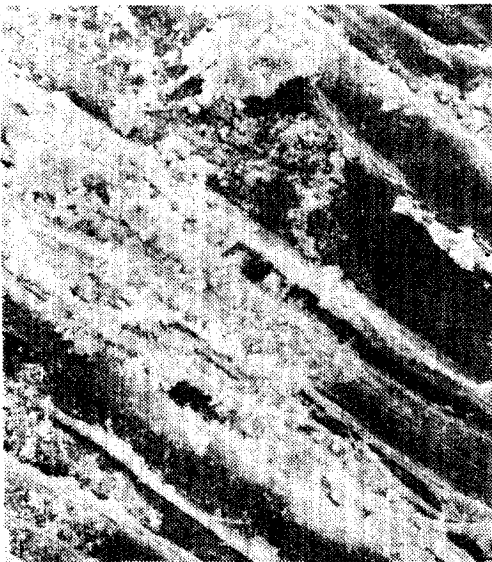
PLATE 7. Scanning Electron Micrographs of a Sliver Surface Showing the Effects of an Accelerator on Cement Setting
