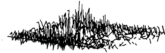
Fig.12. The reconstructed (LSC) image of the cylinder shown in Fig.6. Severe noise, about 200% maximum added to the line integrals, has ruined the impression of a cylinder.
