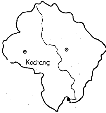
watershed ⊙ rain gage (recording) — main stream ● stream gage Fig. 5 Rainfall and Stream Observation place for Kochang Stream of Inchon River Basin
