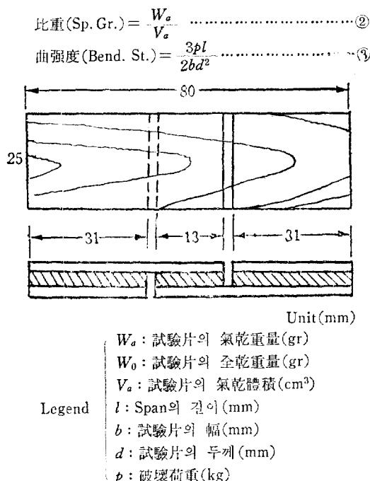
Fig. 1. Test sample of plywood shear strength
