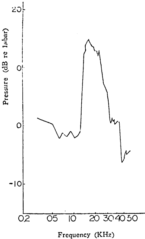
Fig. 8. Sound spectrum of sea noise at moving shackles in water tank.
