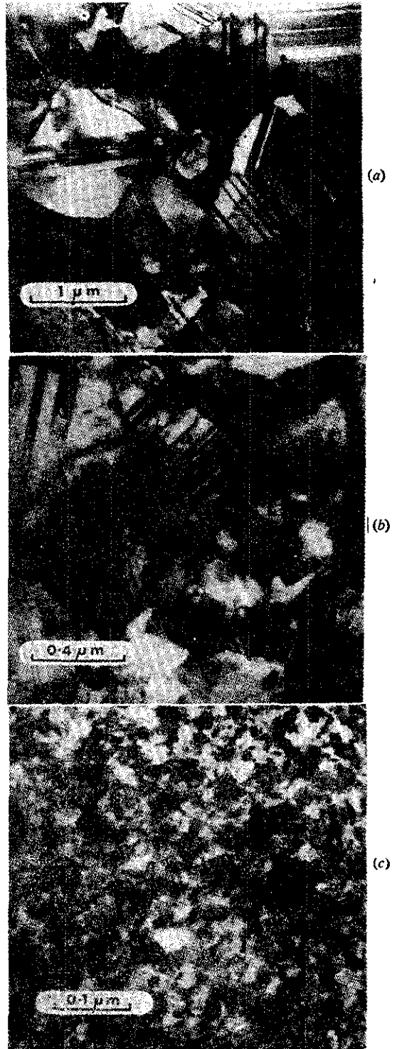
Fig. 6 Transmission electron micrographs of nickel electrodeposits plating conditions: 55°C, pH 4, 4A/dm 2 . (a) Watts nickel; (b) semi-bright nickel; (c) bright nickel.
