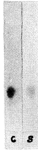
Fig. 7. The spots detected from sample and standard by T.L.C. C: Citrus unshiu , S: Synephrine
