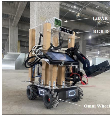
Figure 3. The robot used in this study for on-site data collection.
