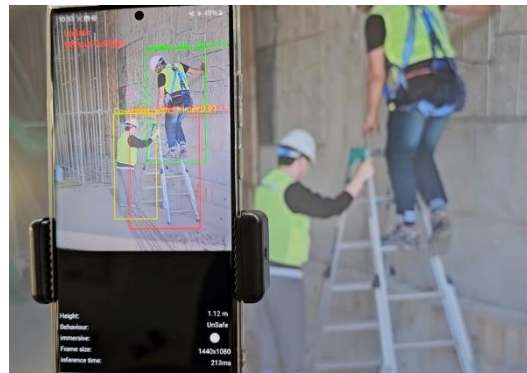
Figure 5 : Realtime mobile application for detecting worker behavior on A-type Ladder
