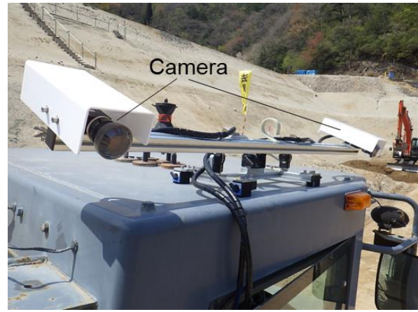
(b) Stereo camera on vibration roller
