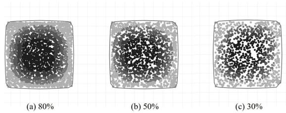
Fig. 6. Surface extraction results for different particle counts.
