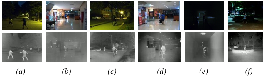
Figure 3. Samples images in the MIHAB dataset. Top row: visible samples, Bottom row: thermal samples. (a) Fighting (Fi), (b) Running (Rn), (c) Biker (Bk), (d) Suspicious Object Carrier (Oc), (e) Bag Left Unattended (Ou), (f) Normal walking pedestrian (No)
