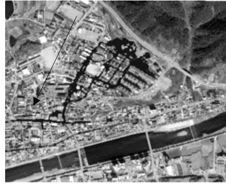
(b) Risk Knowledge Visualization using FLO-2D Spill Simulation Result
