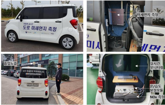
Fig. 1. Road fine dust measurement vehicle and configuration diagram.
