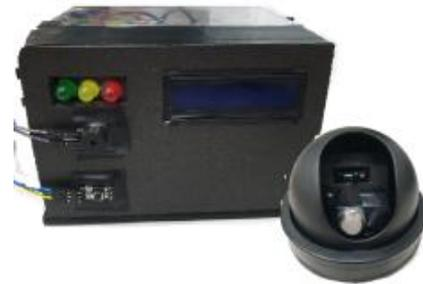
Fig. 4. The Smart Fire Detector
