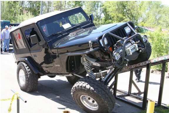
Fig. 1. - Jeep ramping an RTI ramp (WikiMedia)
