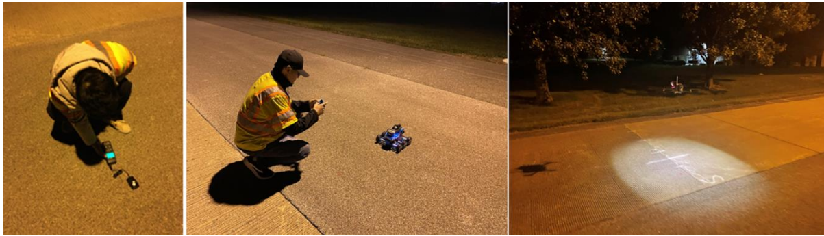
Figure 4. Manual (left), cart (middle), and drone (right) illuminance measurement
