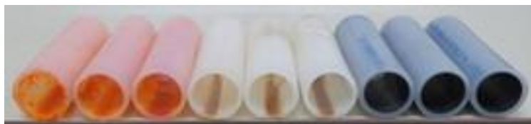
Figure 2. XL pipes contaminated with Contaminant 1 (Left), Contaminant 2 (Center), and Contaminant 3 (Right)
