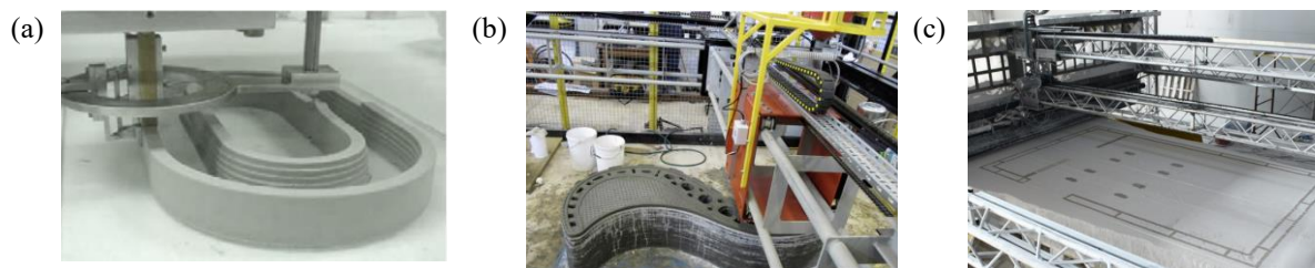
Figure 1. Three typical kinds of concrete 3D printing technologies: (a) Contour Crafting [3], (b) Concrete Printing [5], and (c) D-shape [6]
