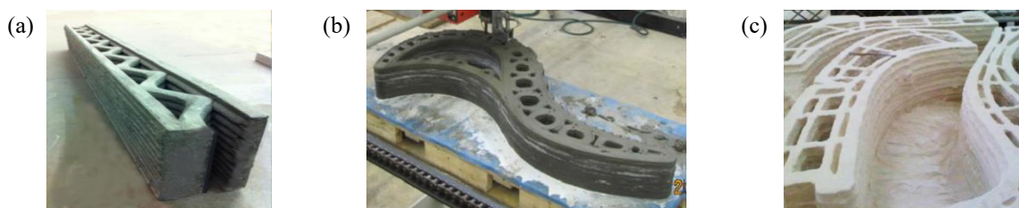
Figure 2. Elements printed by (a) Contour Crafting [7], (b) Concrete Printing [8] and (c) D-shape [6] respectively
