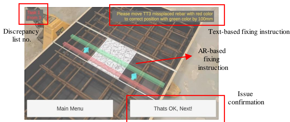
Figure 5. The inspector guiding interface showing a discrepancy of a top transversal rebar
